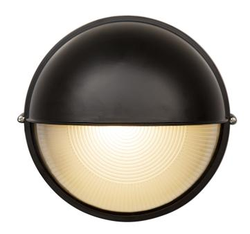
This large round bulkhead is made of durable die-cast aluminium and comes in classic black. The frosted glass lamp shade provides a soft glow, while the E27 lamp base supports up to 100W of power. With an IP54 rating, it's resistant to dust and water. Measuring 240mm in diameter and 125mm in depth, this non-dimmable bulkhead is perfect for outdoor lighting needs.
